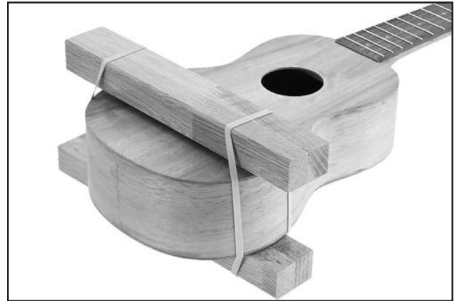
Figure 18. Bridge secured with wood blocks.
