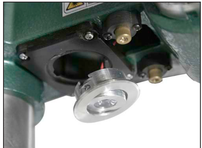
Figure 90. Laser module and LED wiring.
