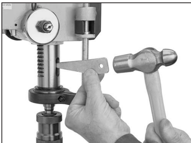
Figure 35. Example of using drift key to remove arbor from spindle.
