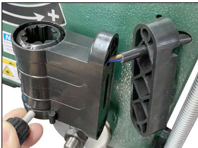
Figure 94. Chip guard micro switch wiring.
