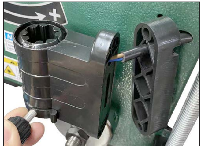
Figure 91. Chip guard micro switch wiring.
