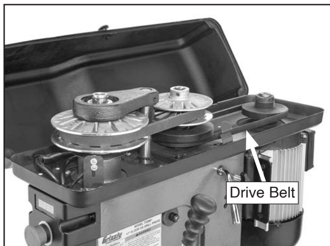
Figure 64. Location of drive belt (T33961 shown).
