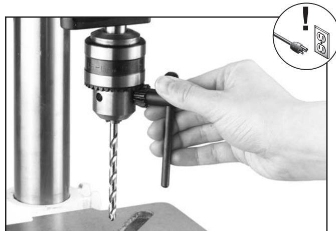
Figure 36. Example of tightening chuck.
