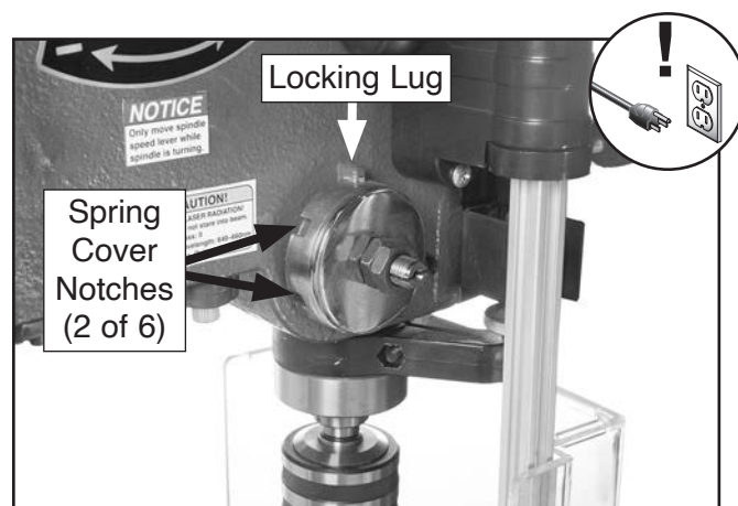
Figure 61. Location of spring cover notches and locking lug (T33960 shown).
