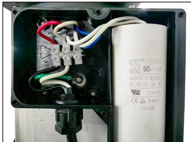
Figure 95. Motor junction box wiring.
