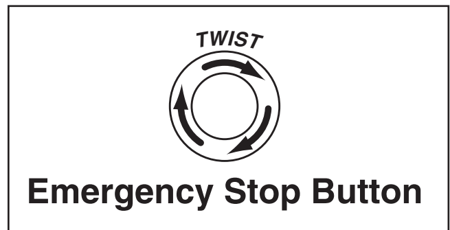
Figure 29. Resetting Emergency Stop button.
