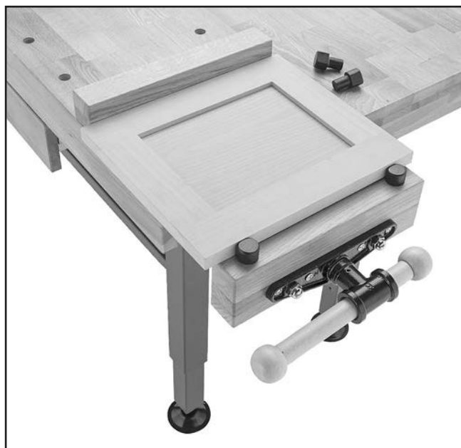
Figure 3. Workbench securing wood project with bench stop, front vise, and bench dogs.
