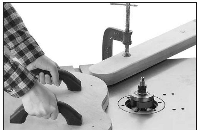
Figure 47. Example of using a template jig with a starting block.
