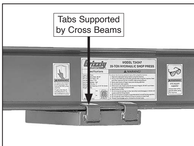
Figure 8. Ram mounting plate tabs supported by cross beams.
