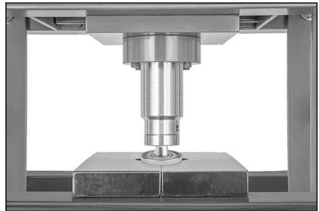
Figure 24. Ram extended to workpiece.
