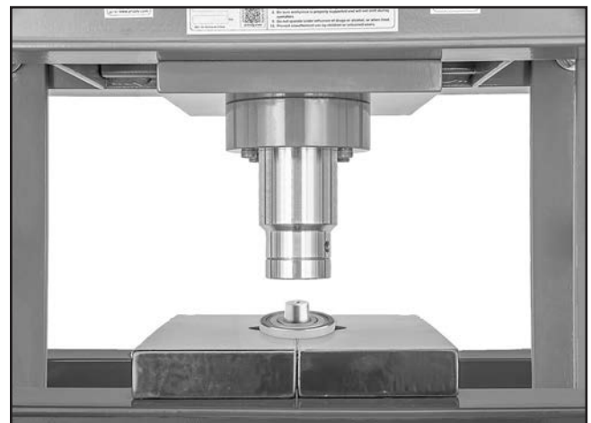
Figure 16. Example of typical hydraulic press operation using V-blocks on press bed.
