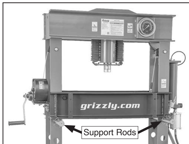
Figure 14. Bed raised to upper operating height.
