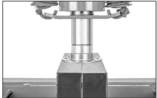
Figure 29. Ram extended to workpiece.
