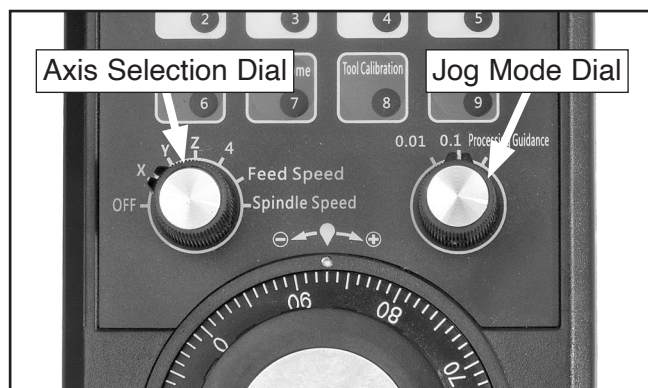
Figure 13. Location of DSP controller axis selection dial and jog mode dial.
