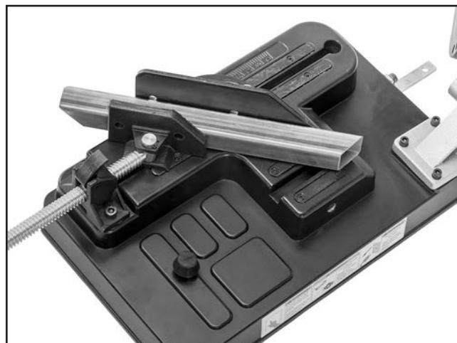
Figure 29. Workpiece secured in vise jaws.
