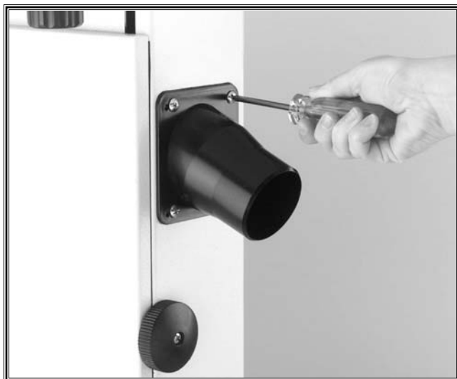
Figure 19. Installing dust port.
