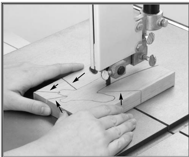
Figure 52. Relief cuts before cutting curves.
