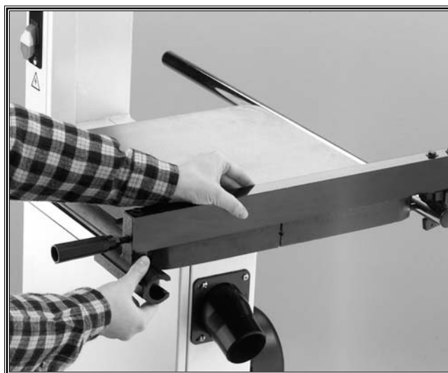
Figure 23. Starting fence on rail.
