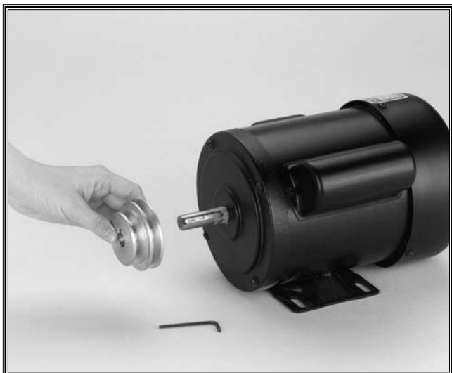
Figure 14. Installing pulley on motor.
