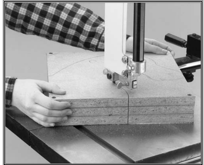
Figure 54. Making a stacked cut.
