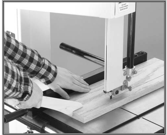
Figure 49. Ripping a board.
