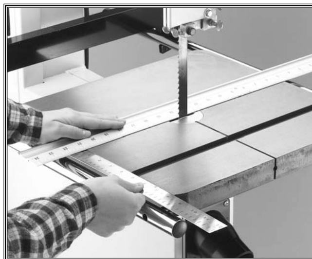
Figure 45. Squaring miter slot to blade.
