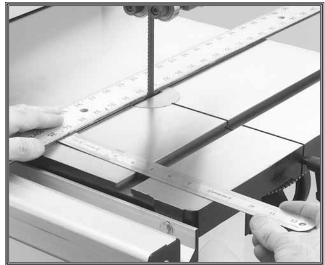
Figure 30. Squaring the miter slot to blade.
