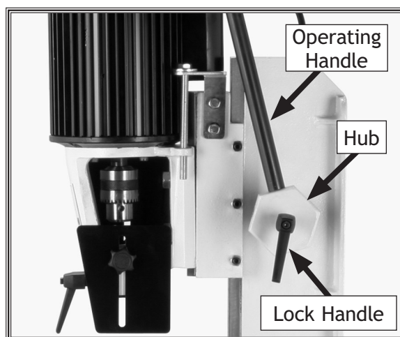
Figure 8. Installing the operating handle.
