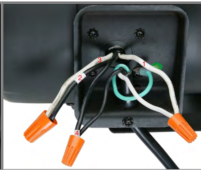
Figure 71. Motor wired for 220V.
