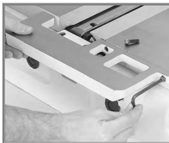
Figure 16. Attaching extension table to jointer.
