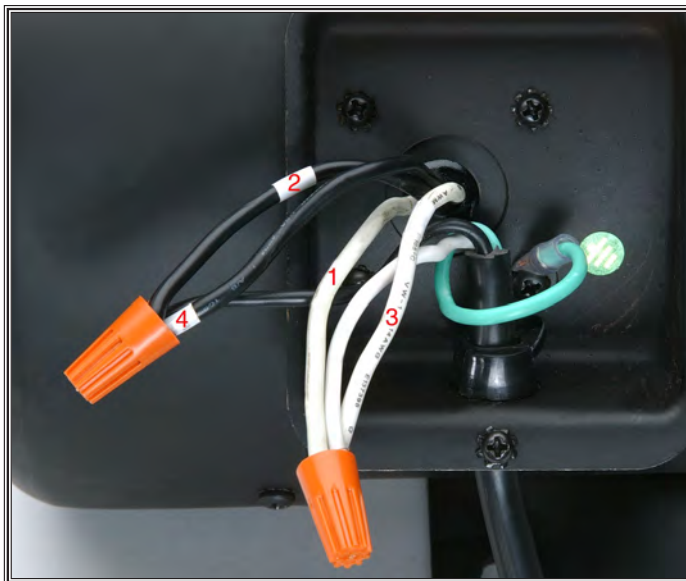
Figure 69. Motor wired for 110V.
