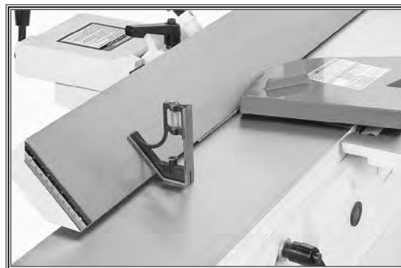
Figure 63. Adjusting fence 45° outward.
