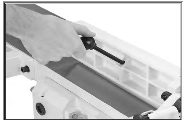
Figure 21. Installing the tilt lever.
