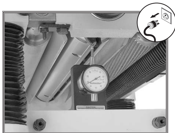
Figure 50. Example of using a Rotacator to find BDC.
