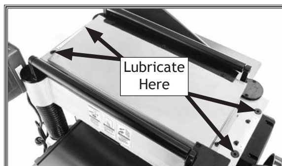
Figure 37. Lubrication locations for feed roller bushings.
