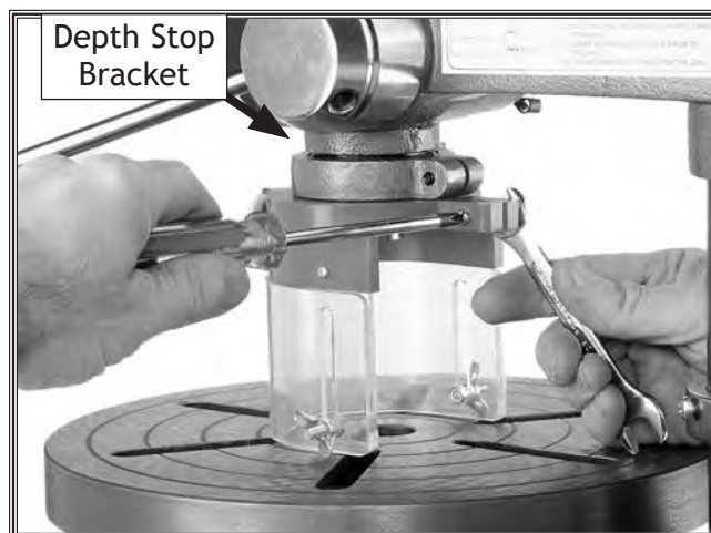
Figure 1. Example photo of installing chuck guard assembly.
